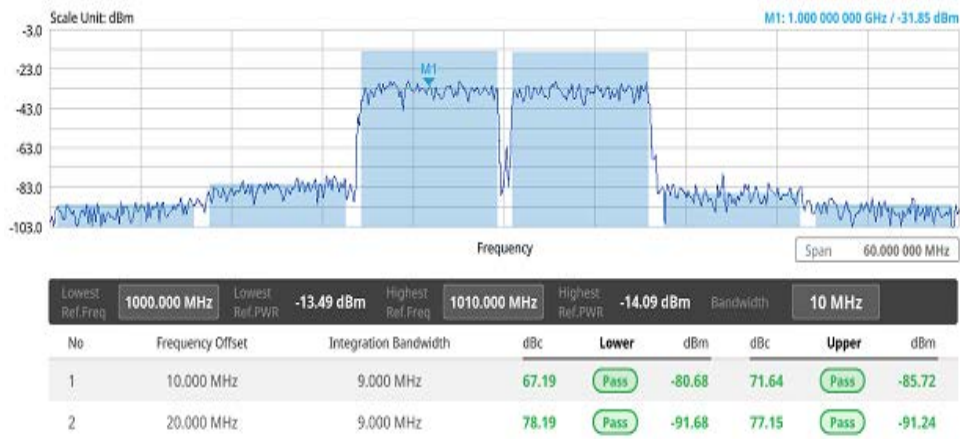
Figure 174 5G DSS Multi-ACLR measurement
