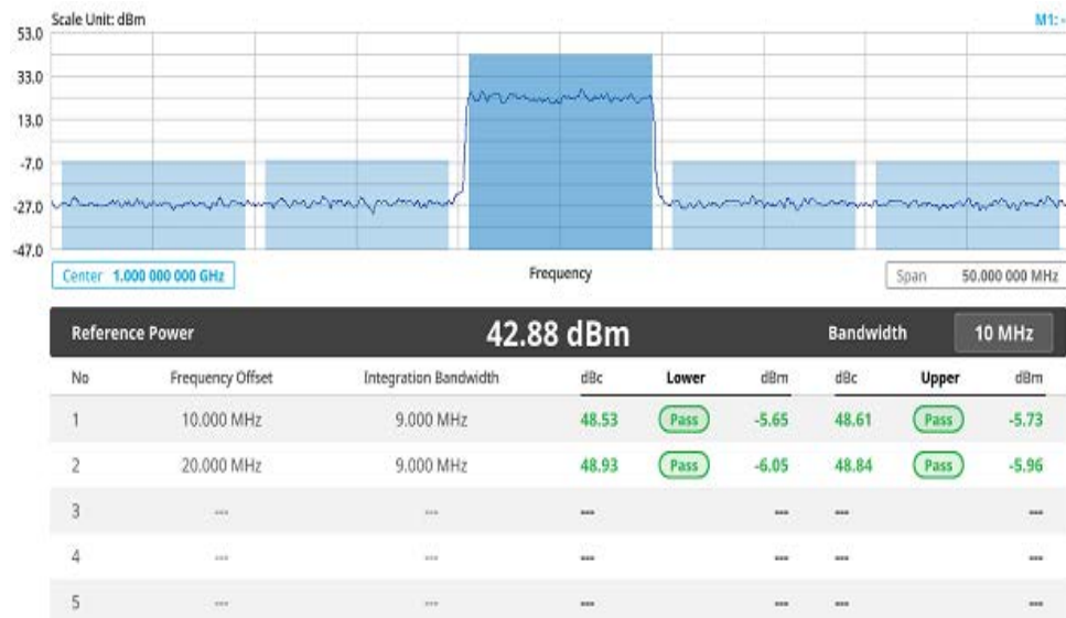
Figure 233 LTE/LTE-A TDD ACLR measurement
