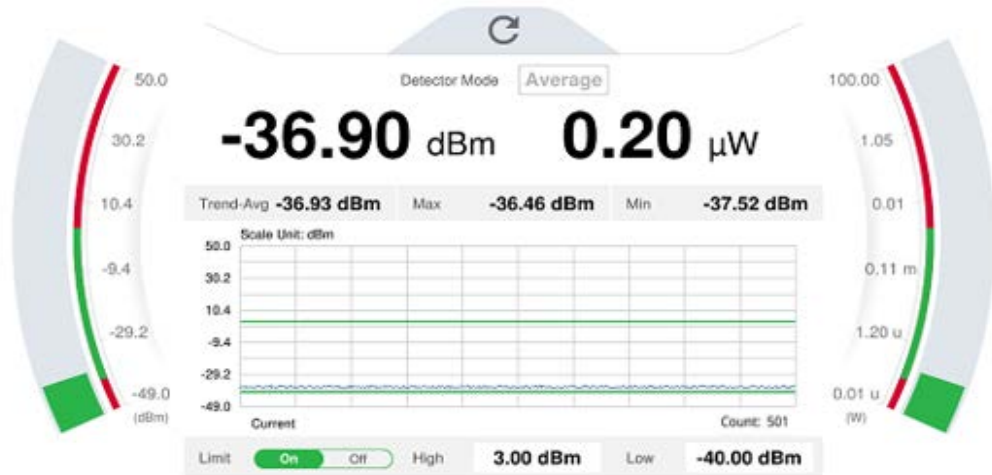
Figure 20 Internal Power Meter with spectrum analyzer
