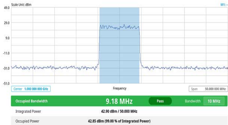
Figure 231 LTE/LTE-A TDD occupied bandwidth measurement
