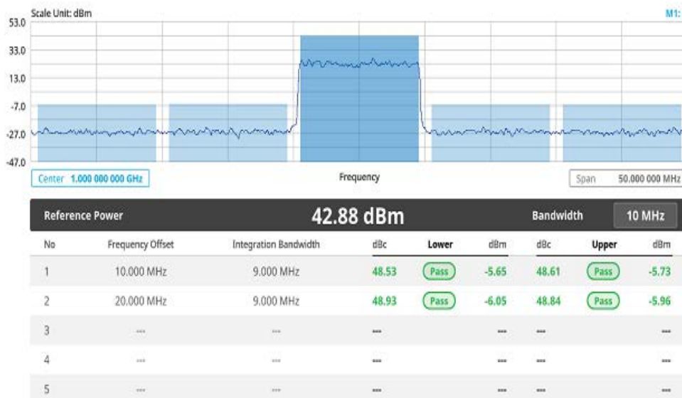
Figure 173 5G DSS ACLR measurement
