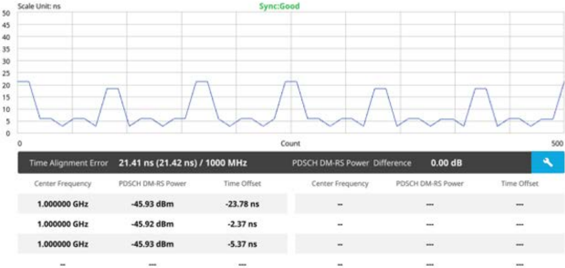
Figure 157 CA time alignment error with 5G TM
