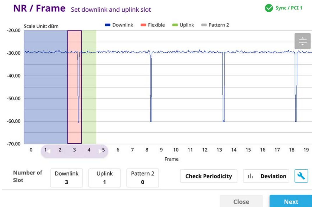
Figure 268 P vs T frame chart view
