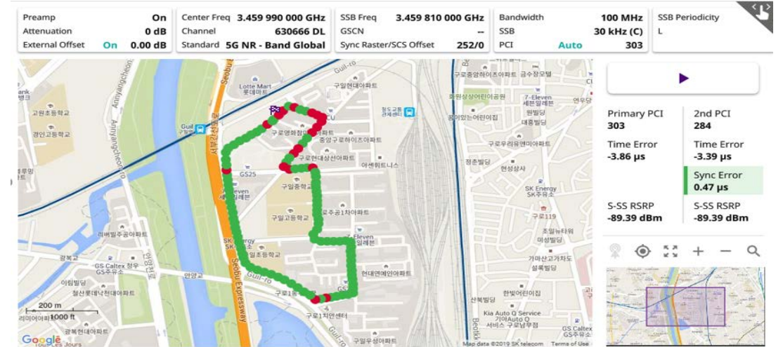
Figure 139 Sync route map with 5G NR Signal Analyzer
