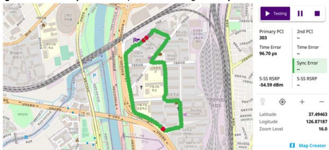
Figure 144 Online sync route map with 5G NR Signal Analyzer
