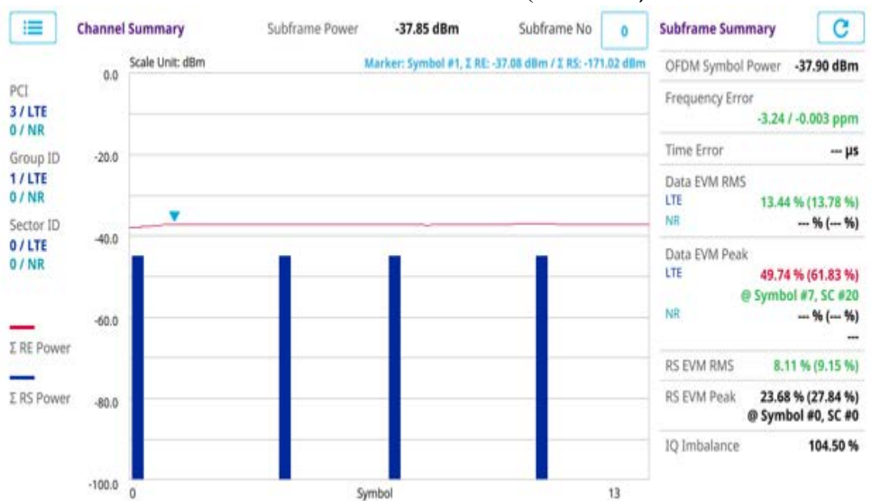
Figure 192 5G DSS DSS subframe measurement (bar chart)
