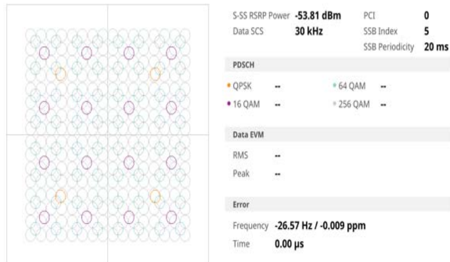
Figure 130 5G NR constellation measurement
