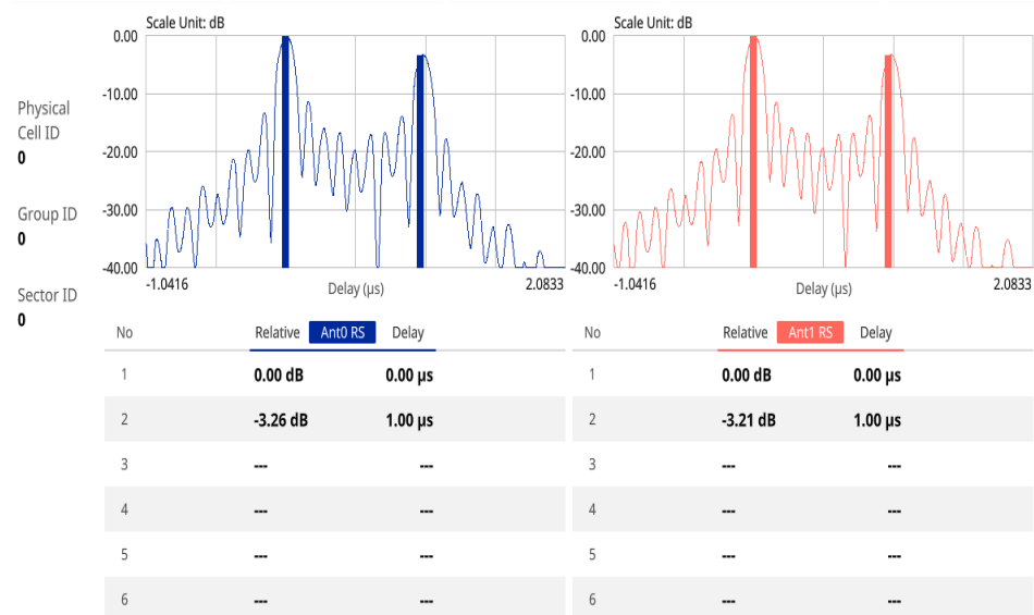
Figure 209 LTE/LTE-A FDD OTA multipath profile measurement
