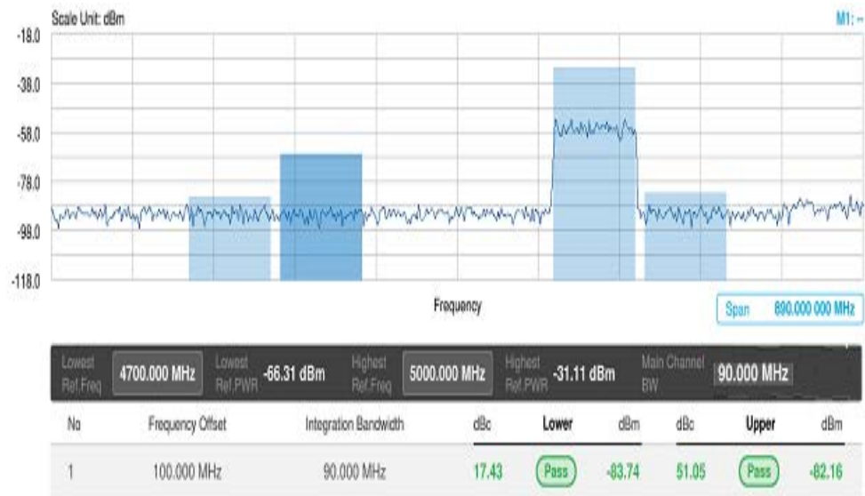
Figure 113 5G NR Multi-ACLR measurement
