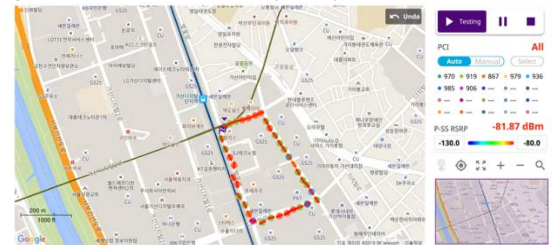
Figure 121 OTA route map with 5G NR Signal Analyzer
