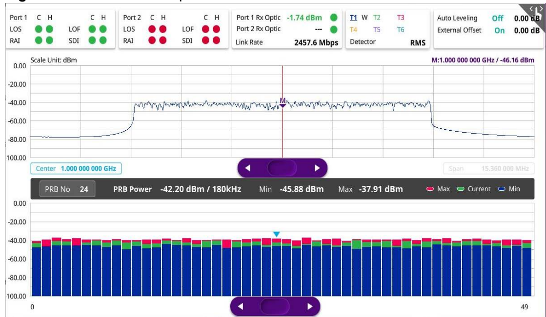
Figure 85 RFoCPRI PRB power
