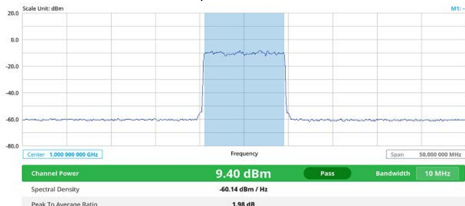
Figure 199 LTE/LTE-A FDD channel power measurement
