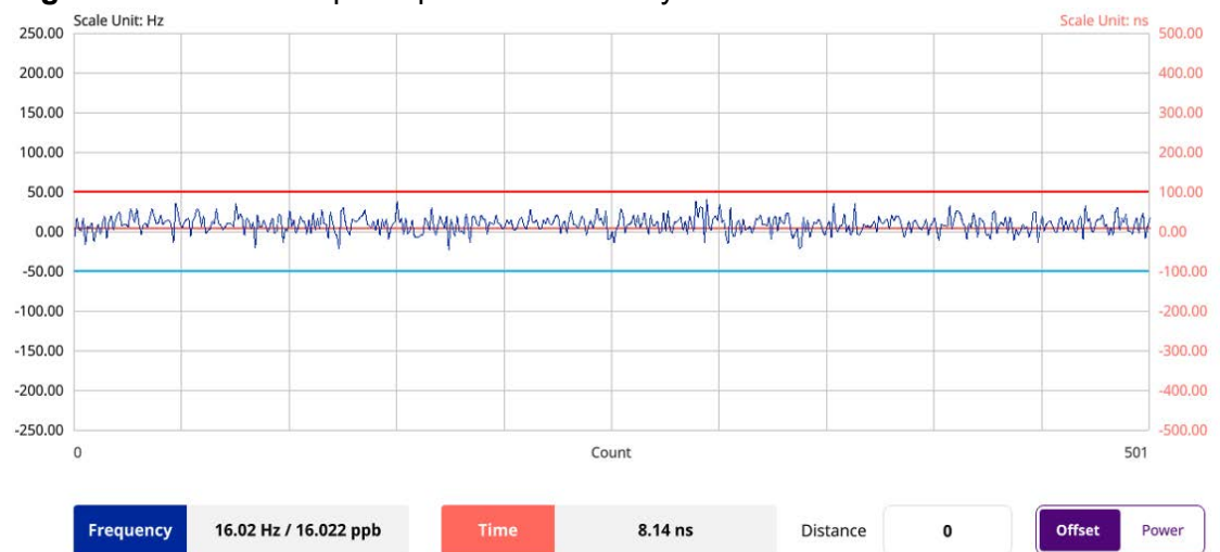
Figure 127 5G NR freq/time/power variation by offset
