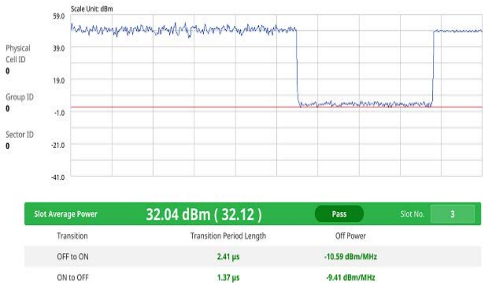
Figure 187 5G DSS Power vs Time (Slot) measurement
