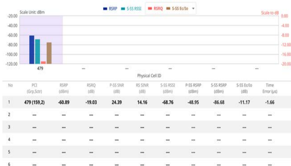
Figure 239 LTE/LTE-A TDD OTA ID scanner measurement
