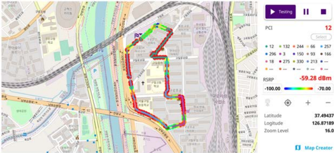
Figure 226 Online OTA Route Map with LTE/LTE-A FDD Signal Analyzer
