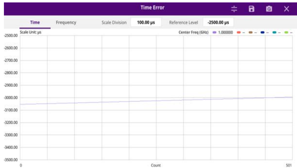
Figure 238 LTE/LTE-A TDD OTA channel scanner with time error
