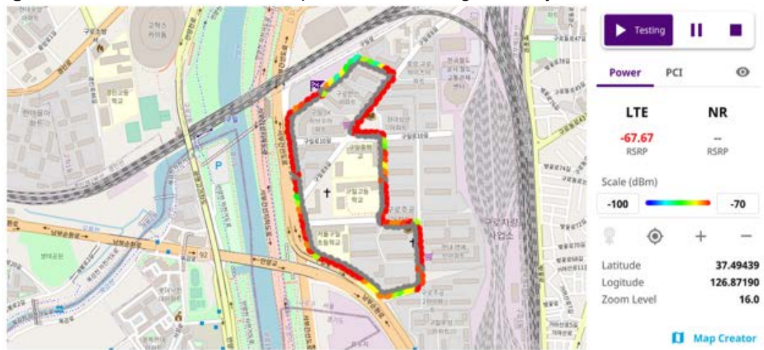
Figure 195 Online OTA Route Map with 5G DSS Signal Analyzer
