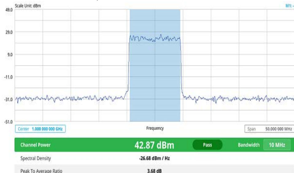
Figure 170 5G DSS channel power measurement
