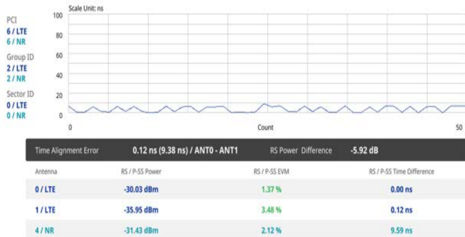
Figure 194 5G DSS DSS time alignment error measurement
