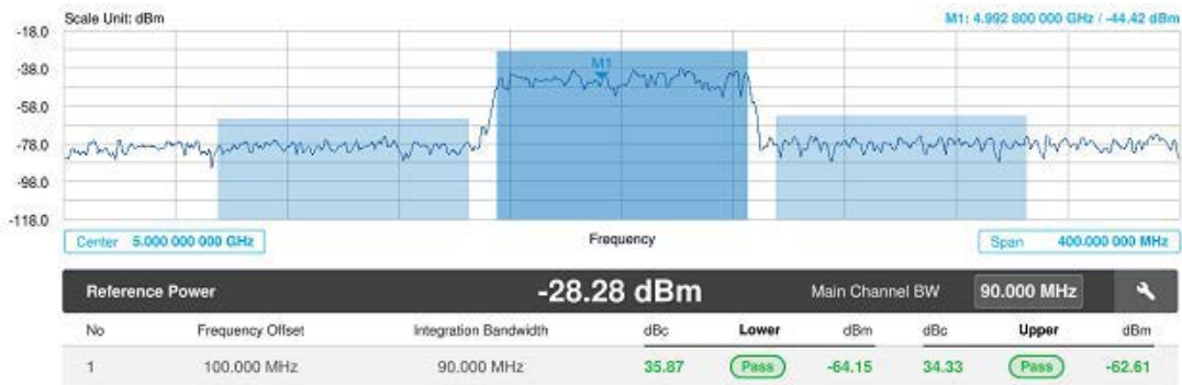
Figure 14 Adjacent channel power measurement with Spectrum Analyzer
