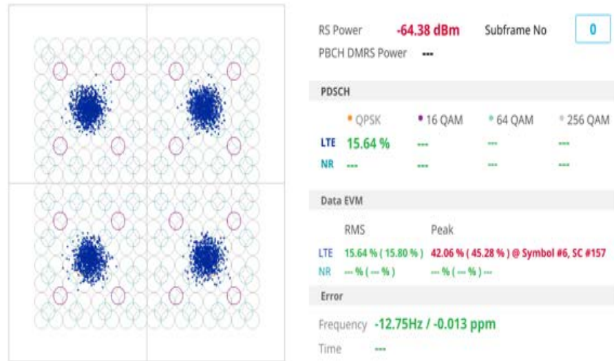
Figure 188 5G DSS DSS constellation measurement
