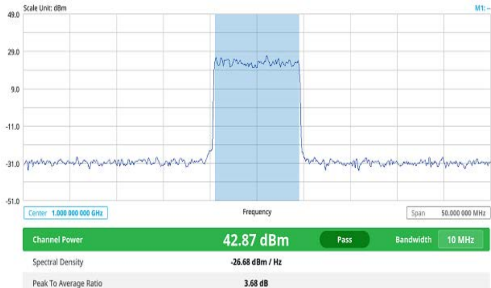
Figure 230 LTE/LTE-A TDD channel power measurement
