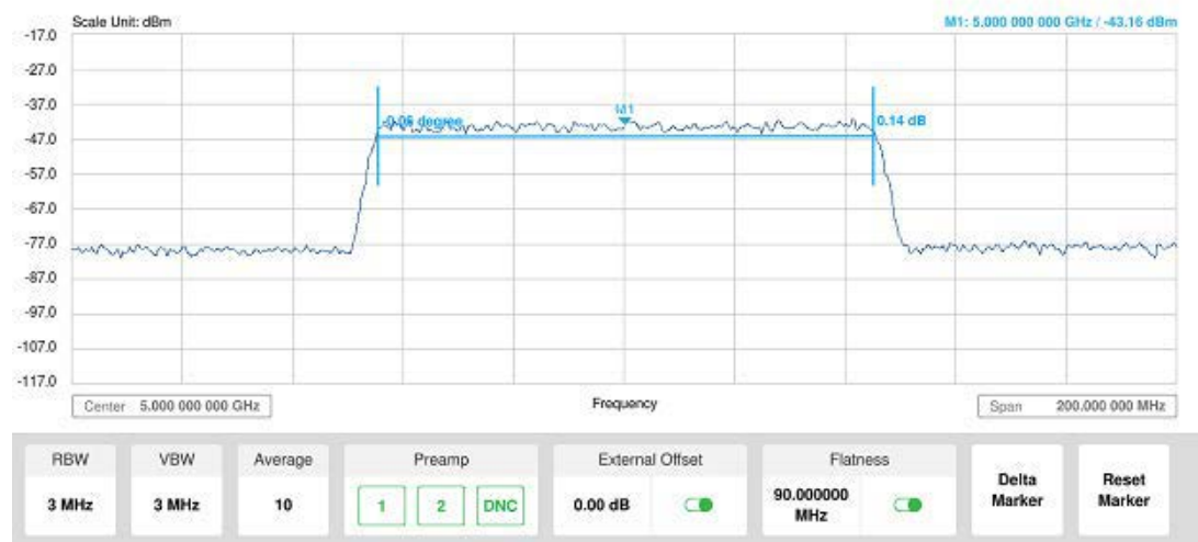
Figure 35 PIM detection — single carrier
