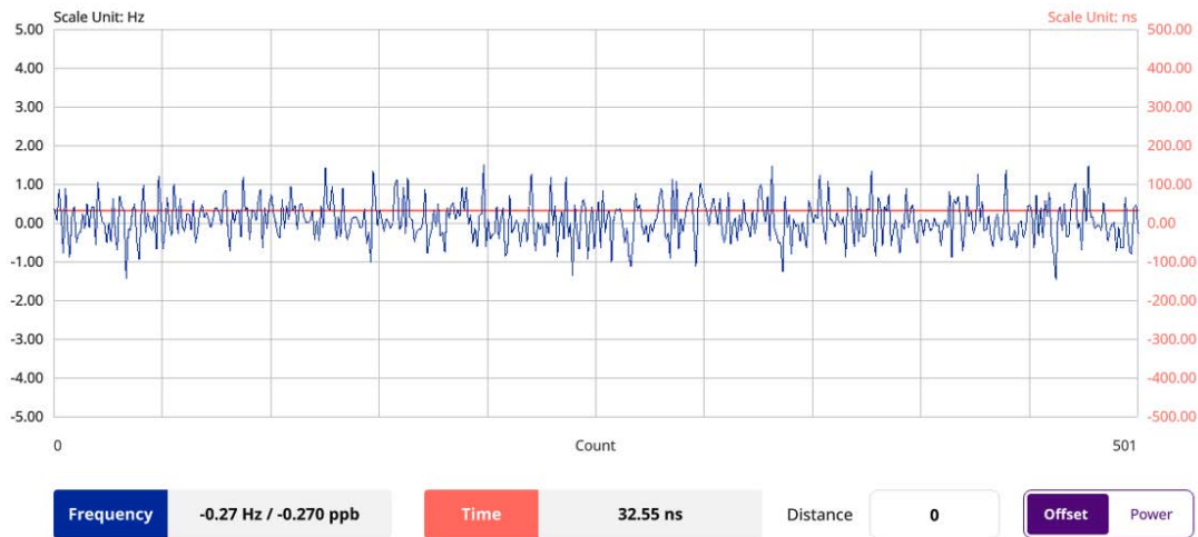
Figure 262 5G NR freq/time/power variation by offset
