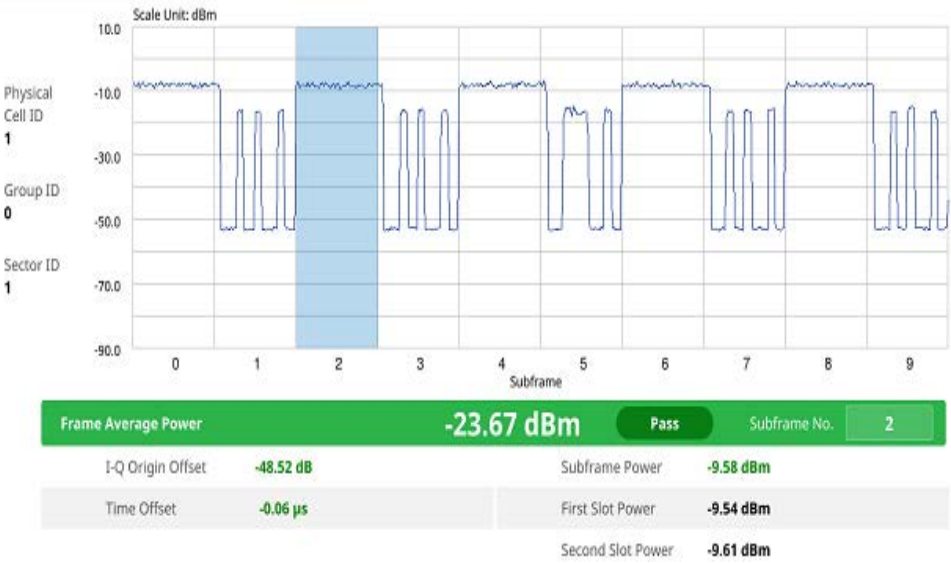
Figure 186 5G DSS Power vs Time (Frame) measurement
