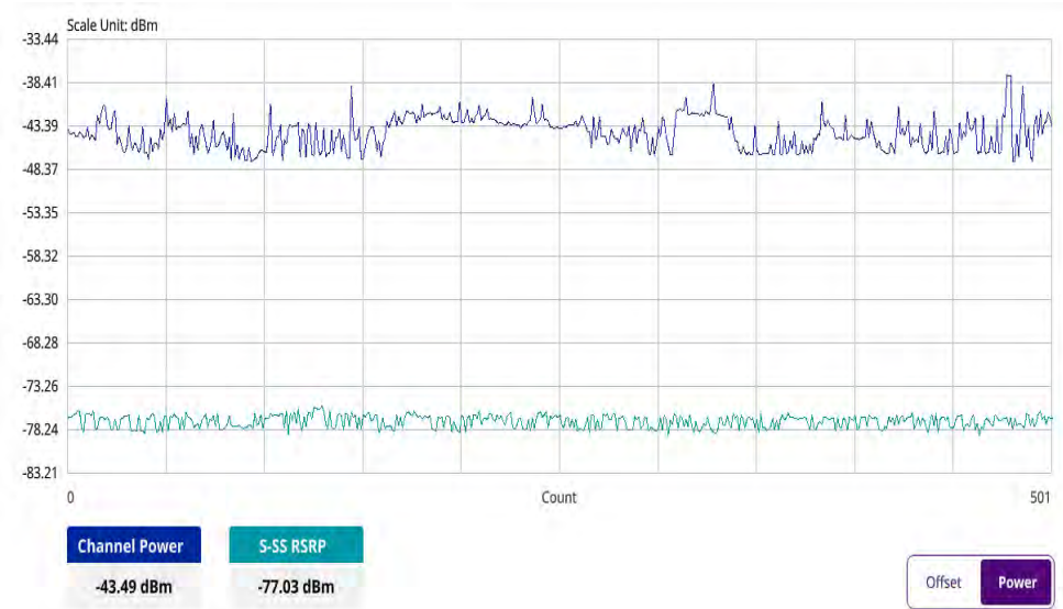
Figure 117 5G NR freq/time/power variation by power
