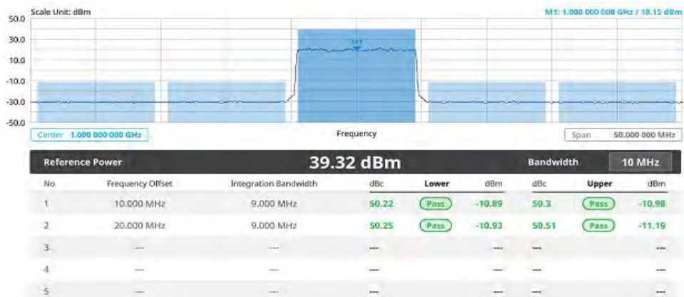
Figure 42 LTE/LTE-A FDD ACLR measurement
