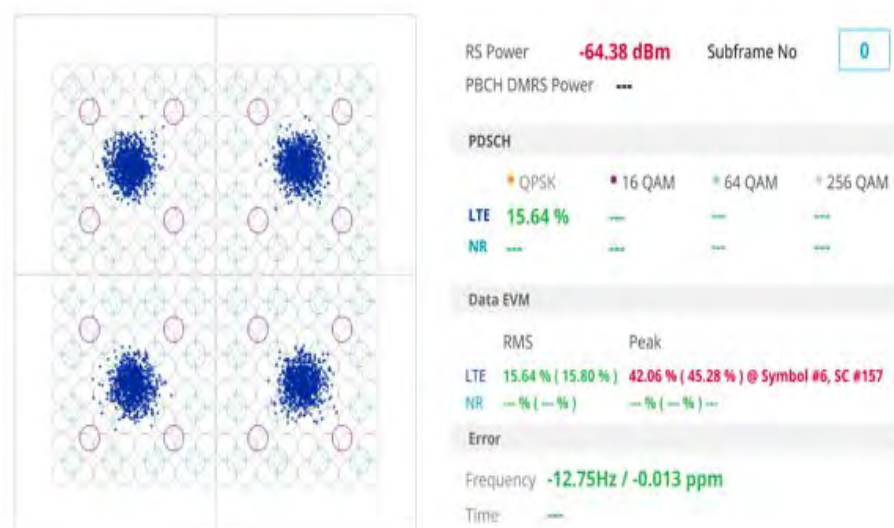
Figure 145 5G DSS DSS constellation measurement
