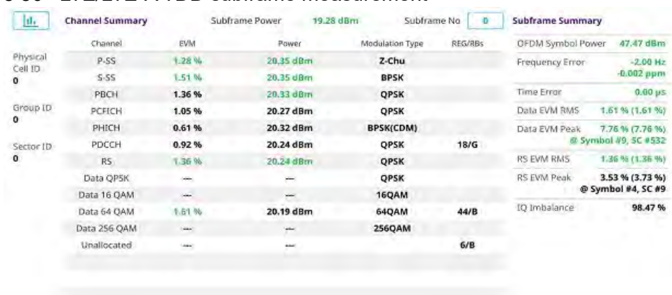
Figure 80 LTE/LTE-A TDD subframe measurement
