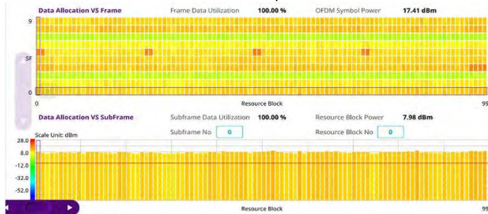
Figure 82 LTE/LTE-A TDD data allocation map measurement
