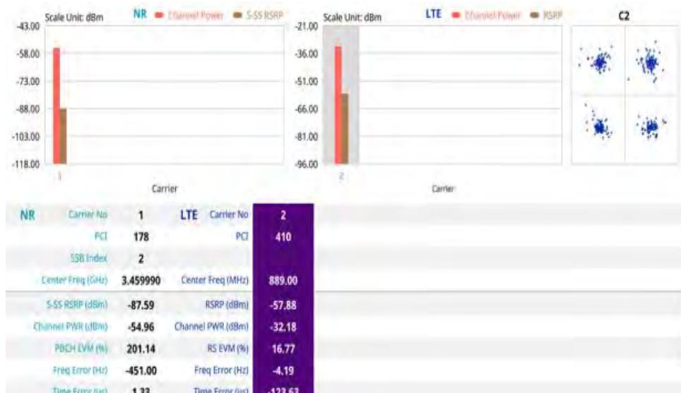
Figure 129 NSA scanner with LTE and NR carrier measurement.
