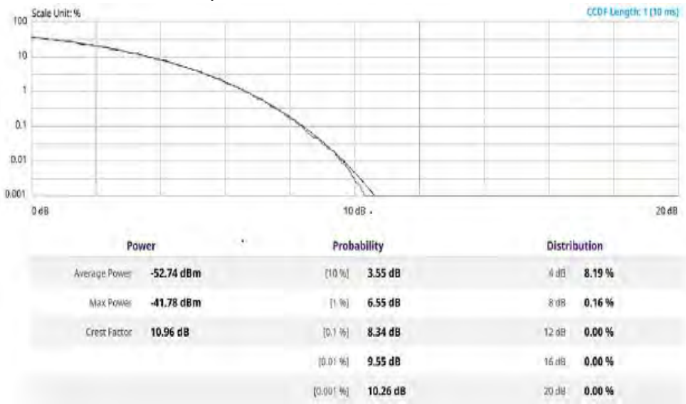
Figure 67 LTE/LTE-A FDD power statistics CCDF measurement
