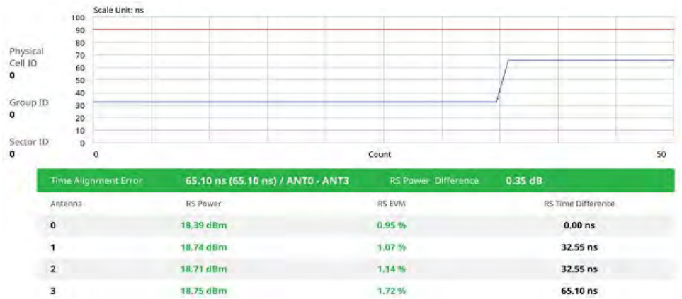
Figure 51 LTE/LTE-A FDD time alignment error measurement
