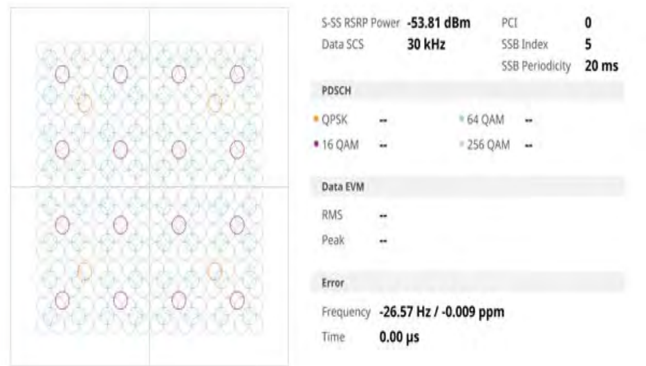
Figure 119 5G NR constellation measurement
