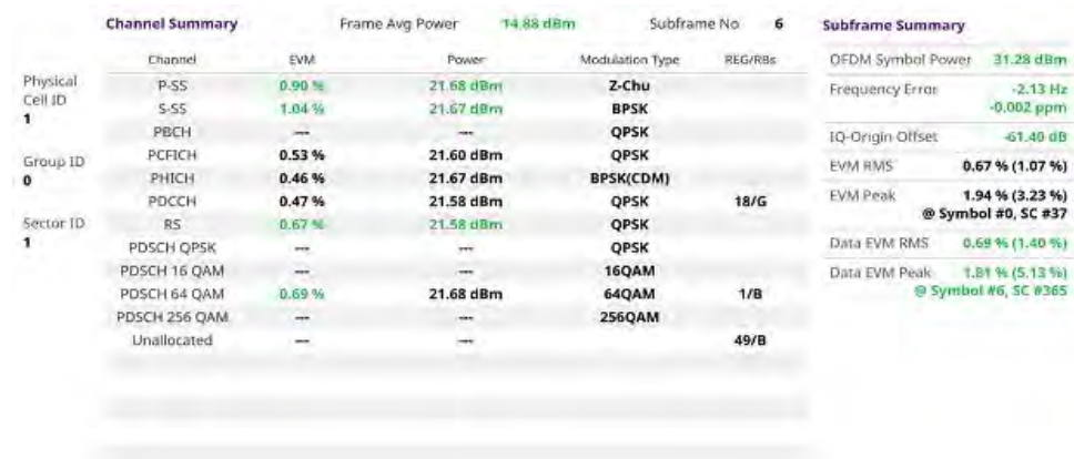
Figure 50 LTE/LTE-A FDD frame measurement
