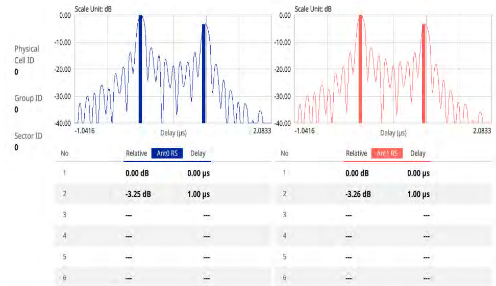
Figure 88 LTE/LTE-A TDD OTA multipath profile measurement
