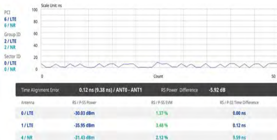
Figure 151 5G DSS DSS time alignment error measurement
