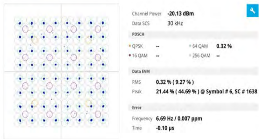
Figure 122 5G NR PDSCH constellation measurement
