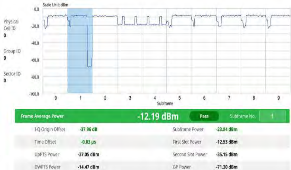
Figure 75 LTE/LTE-A TDD power vs time (Frame) measurement
