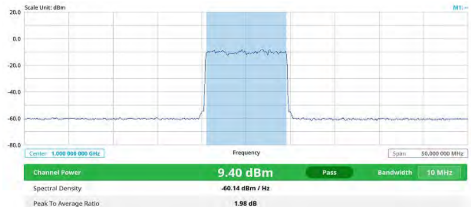
Figure 39 LTE/LTE-A FDD channel power measurement
