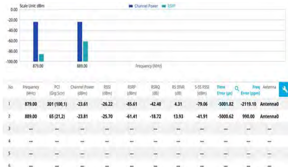
Figure 84 LTE/LTE-A TDD OTA channel scanner measurement
