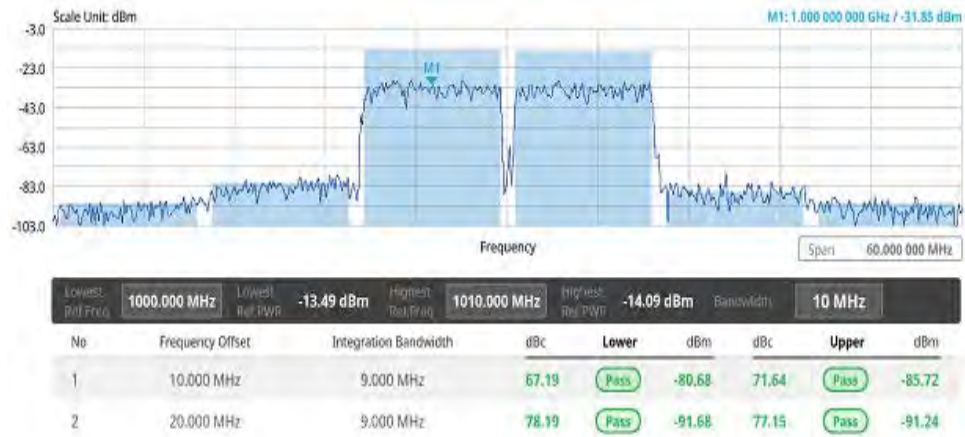
Figure 73 LTE/LTE-A TDD Multi-ACLR measurement
