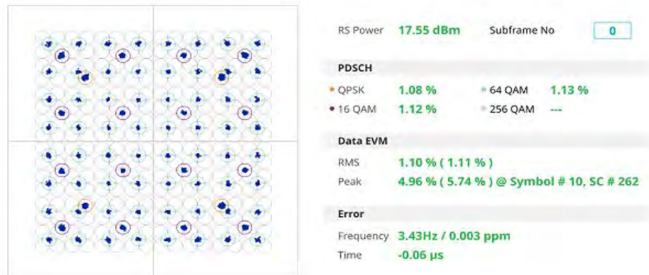
Figure 46 LTE/LTE-A FDD constellation measurement
