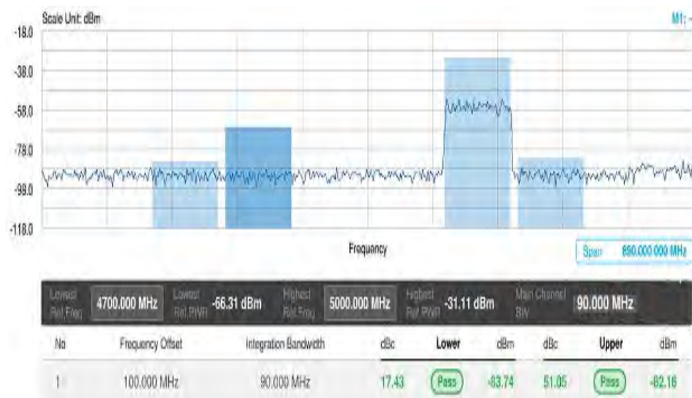
Figure 103 5G NR Multi-ACLR measurement
