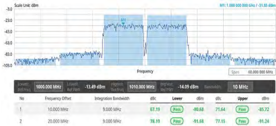
Figure 141 5G DSS Multi-ACLR measurement
