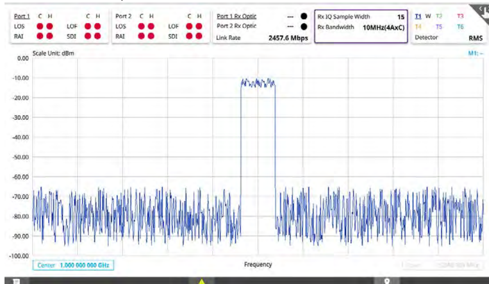
Figure 170 RFoCPRI spectrum measurement (Quad)
