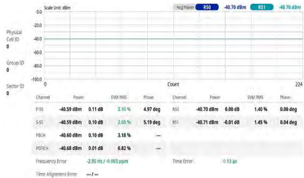
Figure 59 LTE/LTE-A FDD OTA control channel measurement
