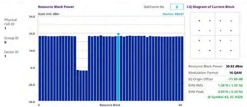
Figure 47 LTE/LTE-A FDD data channel measurement
