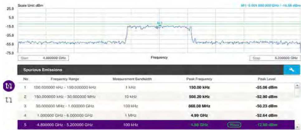
Figure 44 LTE/LTE-A FDD spurious emissions measurement
