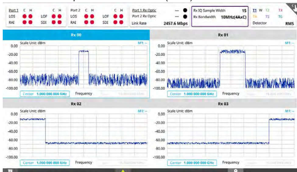
Figure 170 RFoCPRI spectrum measurement (Quad)
