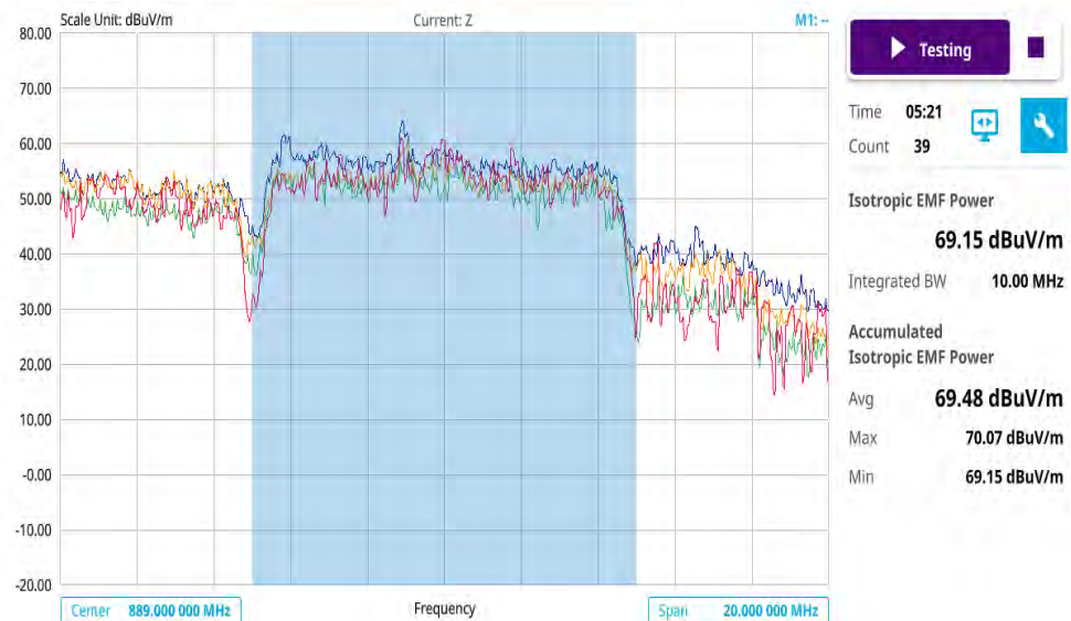
Figure 177 EMF spectrum (level recorder) measurement
