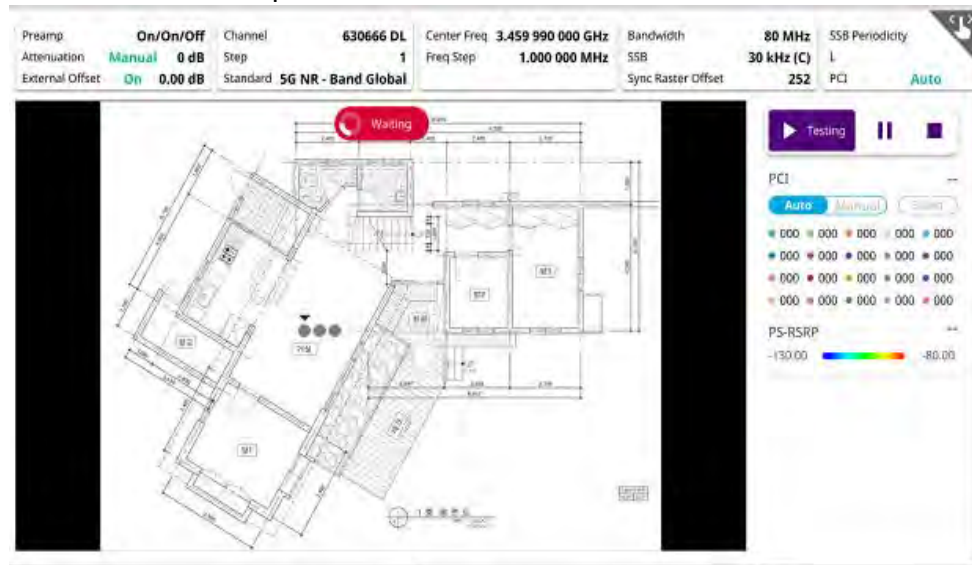
Figure 114 OTA route map measurement with Plot Point to Time
