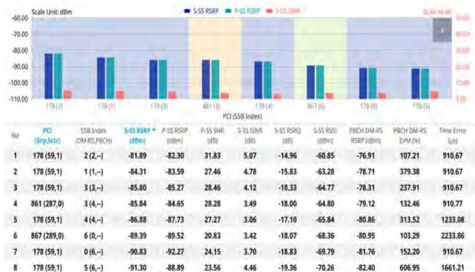
Figure 105 5G NR beam analyzer measurement
