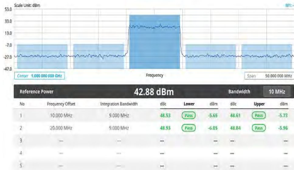
Figure 72 LTE/LTE-A TDD ACLR measurement
