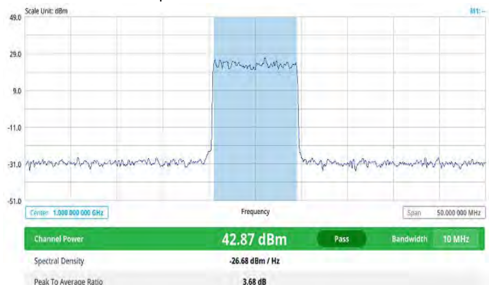
Figure 137 5G DSS channel power measurement
