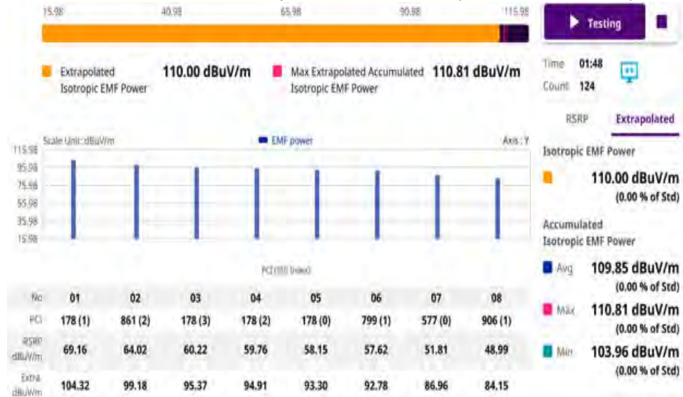
Figure 181 EMF 5G NR beam analyzer measurement (with level recorder)
