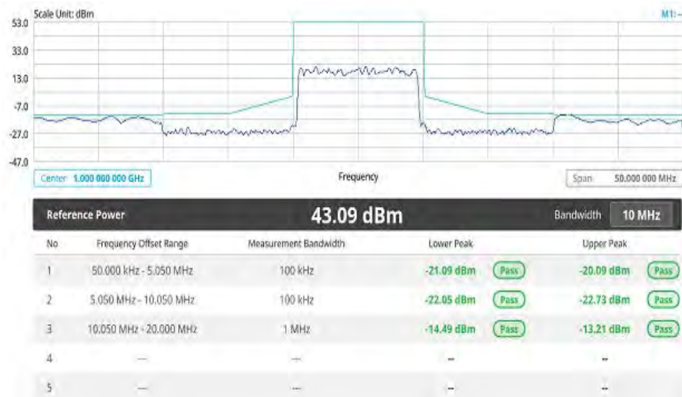
Figure 71 LTE/LTE-A TDD spectrum emission mask measurement
