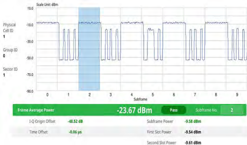
Figure 143 5G DSS Power vs Time (Frame) measurement
