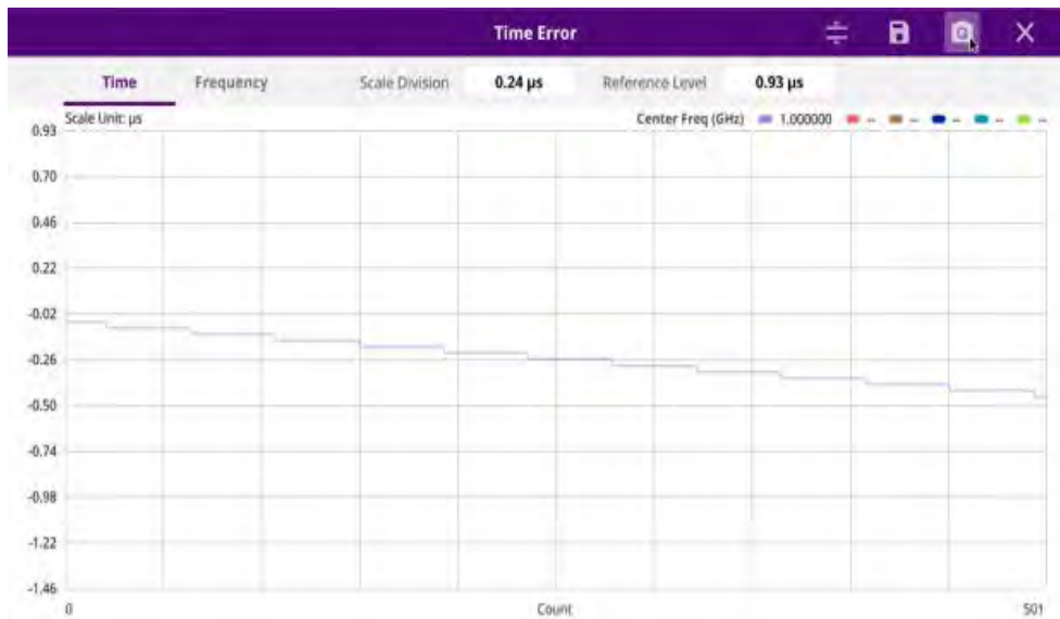
Figure 56 LTE/LTE-A FDD OTA channel scanner with time error
