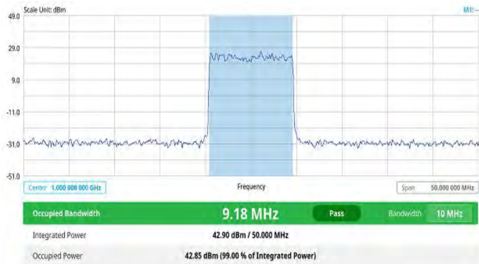
Figure 70 LTE/LTE-A TDD occupied bandwidth measurement
