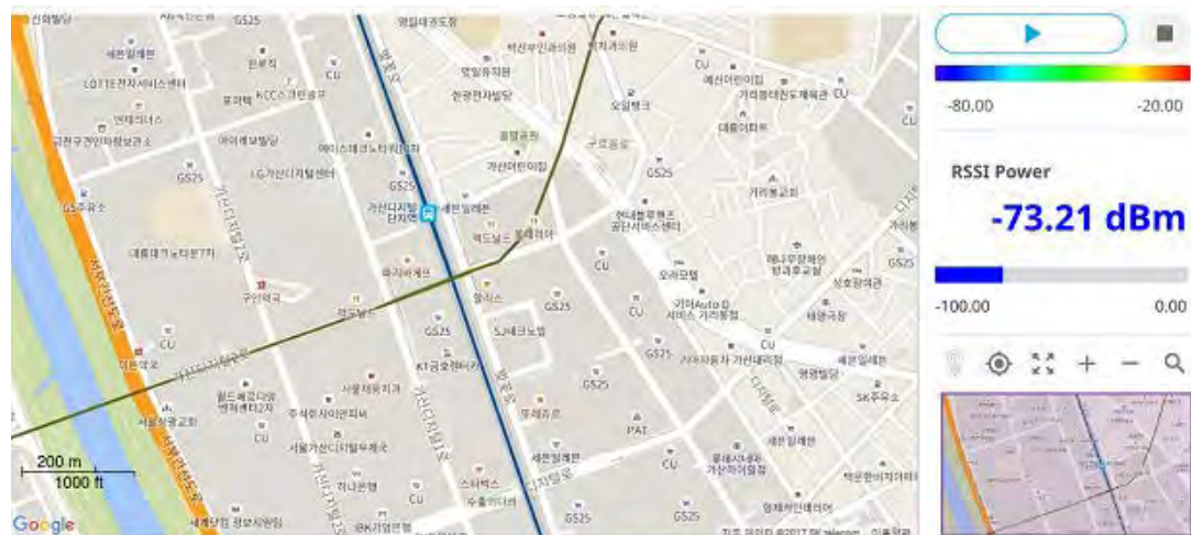
Figure 19 Route Map with spectrum analyzer
