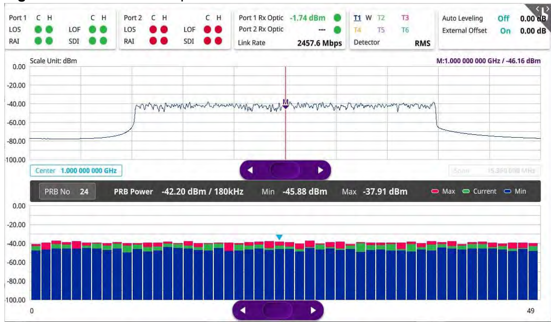
Figure 173 RFoCPRI PRB power
