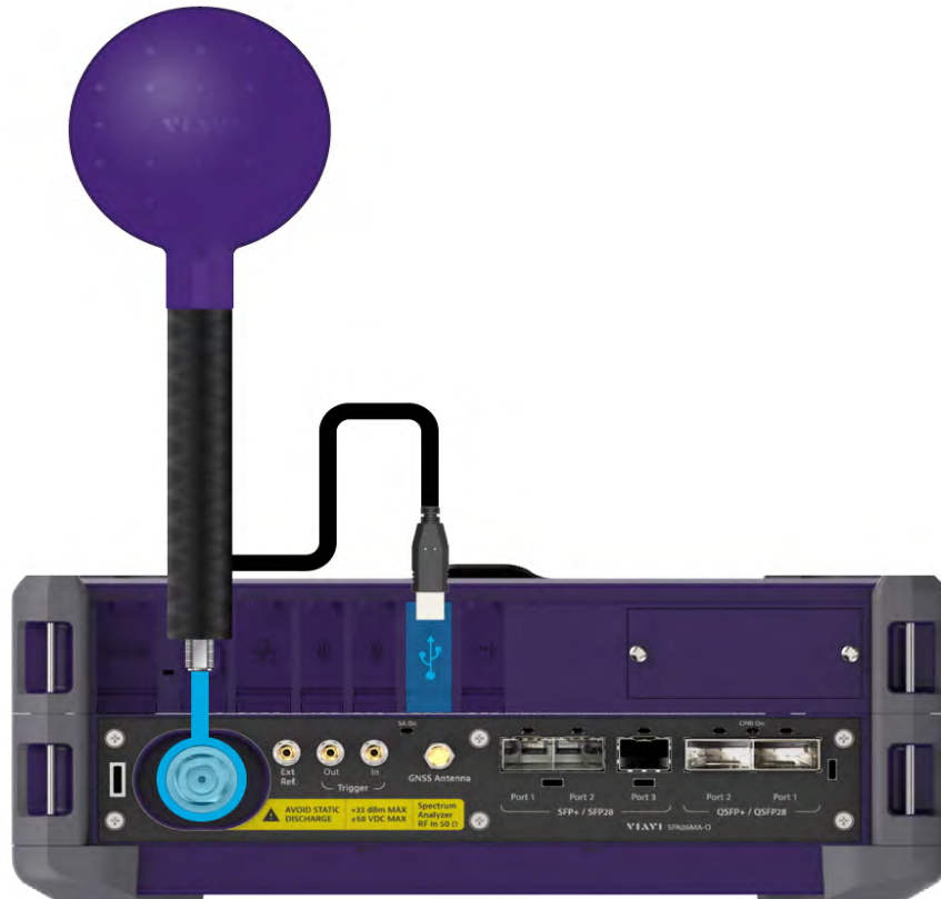
Figure 174 Connecting an isotropic antenna
